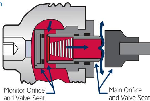
The internal monitor (IM) operates like a standard upstream monitor set, in that the monitor orifice is wide open under normal conditions. Normal regulation and lockup occur at the main valve seat and orifice. (The closing spring causes CL models to lock up at both seats under normal conditions.)
