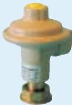
Designed for residential applications from low pressure service lines. WMR can be mounted directly to meter inlet pipe. Its compact angle design makes it specially adequate for installation in space saving meter boxes, indoors or outdoors, or in meter bars.
