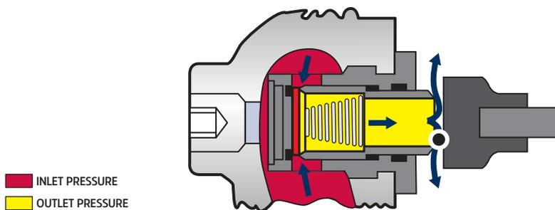
If the regulator fails to control the flow of gas due to foreign matter or damage at the main seat and orifice, the secondary orifice automatically takes control at a slightly elevated outlet pressure. The point of regulation moves to the upstream monitor seat and orifice.
