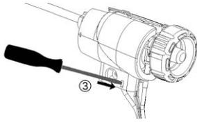
3 Unlock halfshell elements and remove (3).
