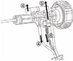
4 Remove adaptor and hose (4), Push thermocouple out of its holder (5) and disconnect cable from thermocouple (6).
