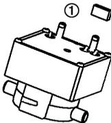
CO measuring cell only: Remove the shorting jumper ①.
