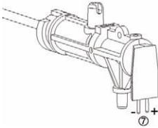
5 Connect lines to the new thermocouple (7, white -, green +) and push thermocouple into holder again.
