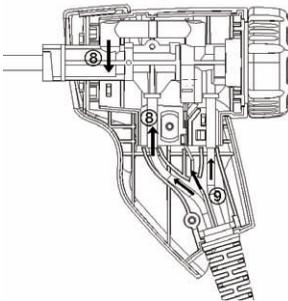
6 Connect adaptor and hose to thermocouple (8). Adjust lines and hoses (9) and attach halfshells.
