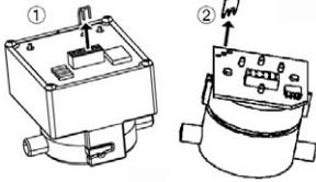
CO measuring cell only: Remove shorting jumper (① 0390 0095, ② 0390 0109).
