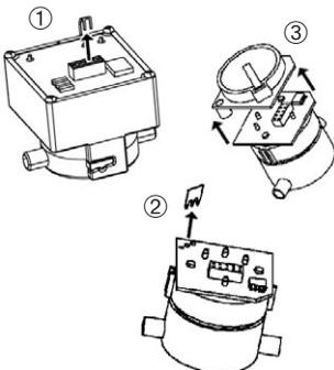
**!** Remove short-circuit brackets/additional boards from the new measuring cells just prior to insertion. Do not leave measuring cells for longer than 15 minutes without short-circuit brackets/additional boards.
