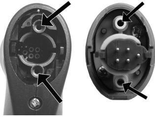
**!** Disconnect the flue gas probe from the measuring instrument prior to cleaning.
