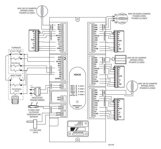
Zone panel wiring—dual fuel: single-stage furnace and single-stage heat pump.
