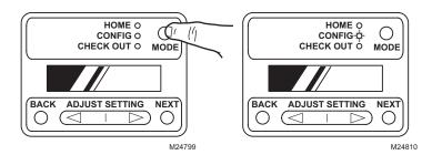
Use the Back and Next buttons to navigate through the configuration menus. Pressing Next enters the selected option for that menu item and advances to the next menu. Adjust settings up or down by pressing the Adjust Setting button.
