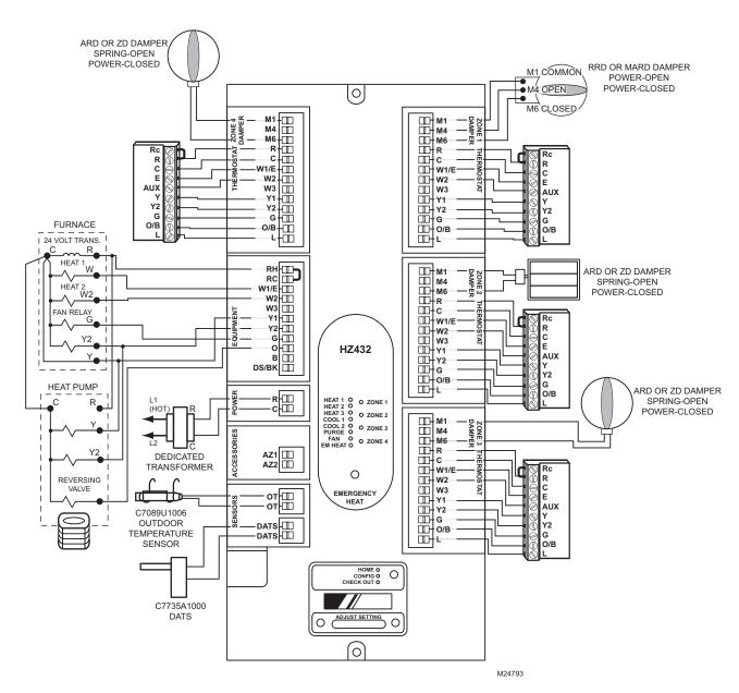
Zone panel wiring—dual fuel: two-stage furnace and two-stage heat pump.
