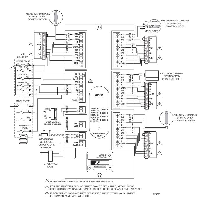
Zone panel wiring—heat pump, 3-heat/2-cool with electric stage 3 heat.
