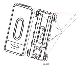
Use two screws for attaching to a stud or roof truss, or four screws for duct or drywall/plaster installations.
