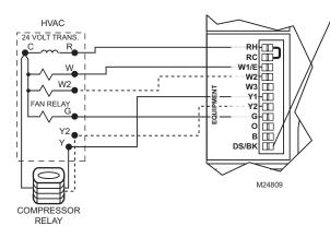
The DS/BK terminal is used with a variable-speed fan. Connect the DS, BK, ODD, or DHUM terminal on the HVAC equipment to this terminal. When 1 zone is calling (or 25% on systems with more than 4 zones) this terminal will be de-energized of 24 VAC. This reduces blower speed on most variable speed blowers.
