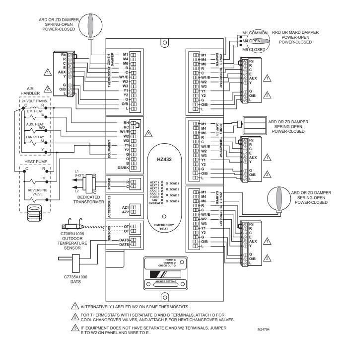
Zone panel wiring—heat pump, 2-heat/1-cool with electric auxiliary heat.
